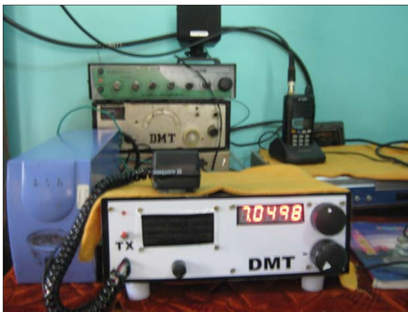
A HAM Radio used in emergency communications is an immensely useful tool for cost-effective dissemination of information
